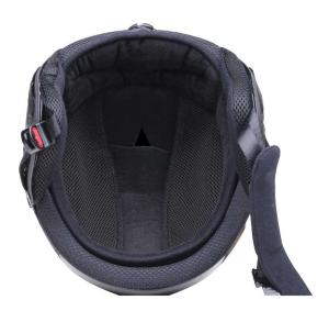
Nevo's comfort lining, comprising a cap in Shalimar, is fixed to the polystyrene inner shell by means of a series of Velcro strips. It is easy to remove. Just ensure that you detach the Velcro strips by holding and pulling the strips themselves. Don't just pull the inner cap out from the helmet.
